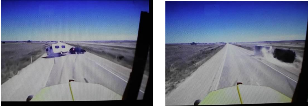
Event No. 7. Tow vehicle braking skid marks turn to yaw marks. Left wheel of caravan starts yaw mark. Car broadsides off road, left wheels drop down embankment, digging in and causing vehicle to roll, caravan roll follows.
