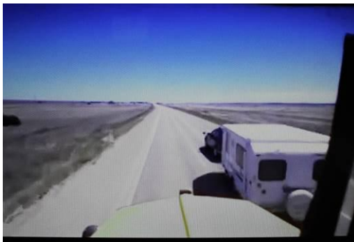
Event No. 5. Caravan releases from bow wave, swinging back towards the front of the truck.
