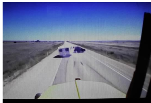
Event No. 6. Harmonic motion swings van from side to side. The black skidmarks are from the car braking hard. There are no caravan braking skidmarks, only yaw marks as the caravan swings back to the left. Driver has totally lost control.
