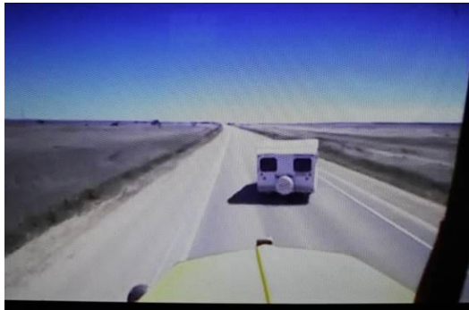
Event No. 5. Caravan releases from bow wave, swinging back towards the front of the truck.
