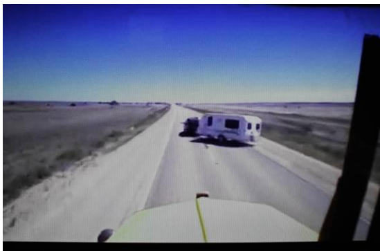
Event No. 6. Harmonic motion swings van from side to side. The black skidmarks are from the car braking hard. There are no caravan braking skidmarks, only yaw marks as the caravan swings back to the left. Driver has totally lost control.
